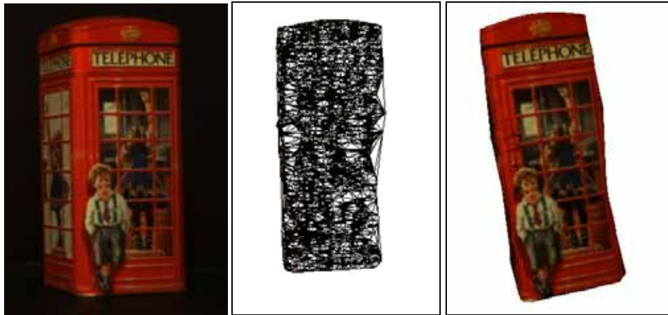
Figure 8: Image (left), 3D mesh (centre), textured model (right) of different models build with the ARCO Object Modeller
